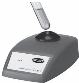
Fig. 21.6 Example of a vortex mixer. The test tube is gently engaged with the orbitally vibrating rubber holder to impart a spinning motion to the liquid within. In some models, the holder can be replaced by an insert for operation with multiple sample vials, e.g. Eppendorf tubes.
