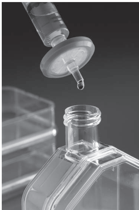
Fig. 21.8 Using a sterile filter. In this example, the Millipore® filter is attached to a plastic syringe, used to take up and expel the liquid.
