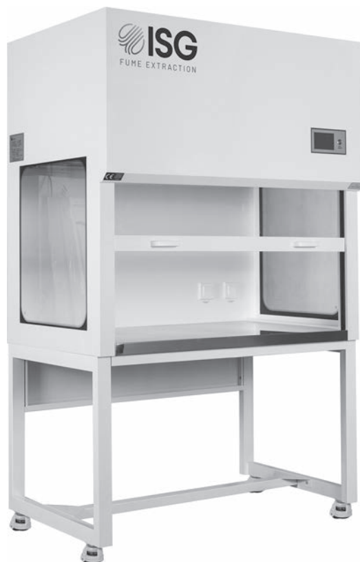
Fig. 33.4 A laminar flow cabinet. Air is drawn in and through a HEPA filter in either the back or the top, exiting the front through the opening created by the moveable glass door. When in use, raise door only enough to enable you to work on the workbench.
