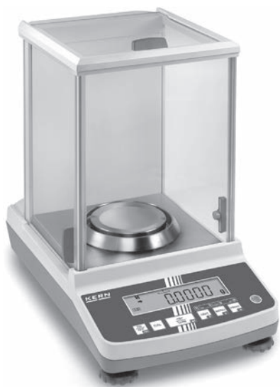
Fig. 21.2 Example of a self-taring electronic balance. Note the shield to help stabilise readings by reducing air flow around the machine.
