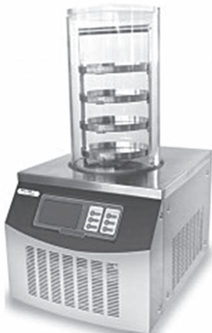
Fig. 21.10 Example of a bench-top freeze dryer, the BioLAB BFBT-101-B. Larger models allow bulk processing and the treatment of bigger specimens. Photo courtesy of Biolab Scientific Ltd.
