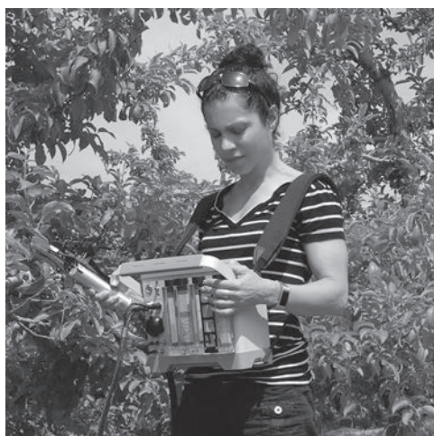
Fig. 64.2 A portable infrared gas analyser, used to measure photosynthetic \text{CO}_2 uptake (leaf cuvette/probe shown in left hand, with analysis unit and user interface below).
