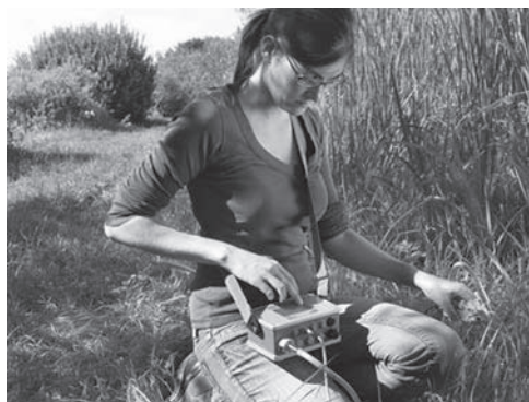
Fig. 64.4 A pulse-amplified modulated fluorometer (PAM), used to measure chlorophyll fluorescence (probe shown in left hand, attached to leaf, with analysis/recording unit on shoulder strap).
